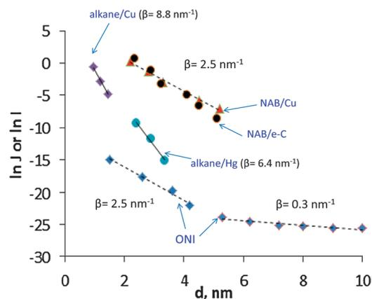
**Fig. 9** Selected attenuation plots for aromatic and aliphatic molecules in ensemble molecular junctions. NAB = nitroazobenzene on carbon with Cu<sup>69</sup> or e-beam carbon<sup>71</sup> contacts, ONI = oligonaphthalene-fluorene-imine on Au using CP-AFM.<sup>67</sup> Y axis is the natural log current density ( $\text{A cm}^{-2}$ ) except for the ONI data which is stated as current due to unknown device area. Alkane/Au and alkane/Hg data are from ref. 37 and ref. 116, respectively.
