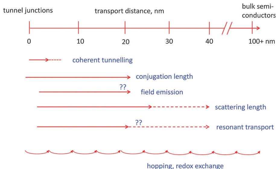
**Fig. 12** Characteristic length ranges for transport mechanisms possible in molecular junctions, from a few nm tunnel junctions to bulk films >50 nm thick where transport is primarily by a hopping mechanism. Dashed lines and question marks indicate that the phenomenon can occur over a range of distances depending on the material and conditions involved.
