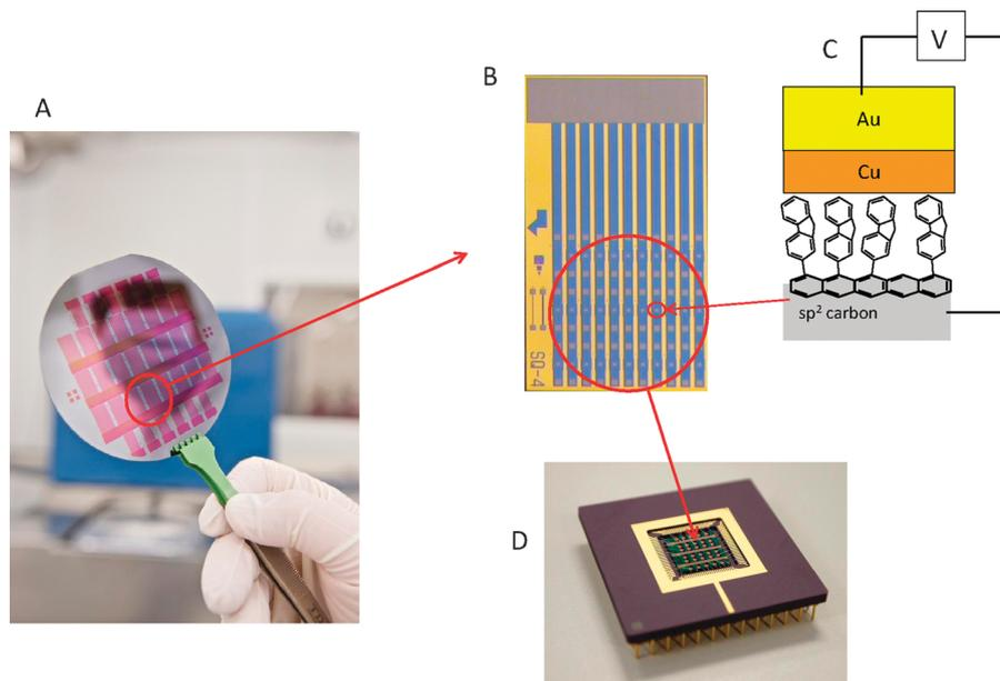
**Fig. 11** Several steps in parallel fabrication of carbon/molecule/Cu/Au ensemble molecular junctions. (A) A 100 mm Si/SiO<sub>2</sub> wafer after photoresist patterning and pyrolysis; (B) individual chip with 32 junction “pads” and contact areas; (C) schematic of a fluorene molecular junction; (D) completed chip after packaging. Details are in ref. 5.
