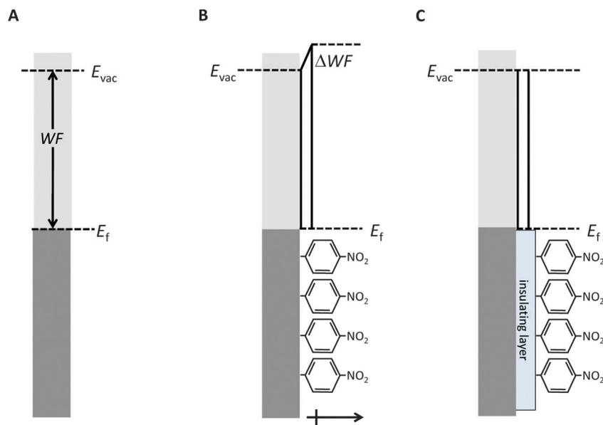
**Fig. 7** Effect of surface modification on the energetics of an interface between a conductor and a molecule. (A) Fermi level and work function of a bare metallic surface in vacuum. (B) Effect of bonding a nitrophenyl layer to the conductor surface. (C) Effect of preventing electronic interactions between the conductor and nitrophenyl layer. Dark gray regions represent filled electronic states in the conductor, light gray is empty states.
