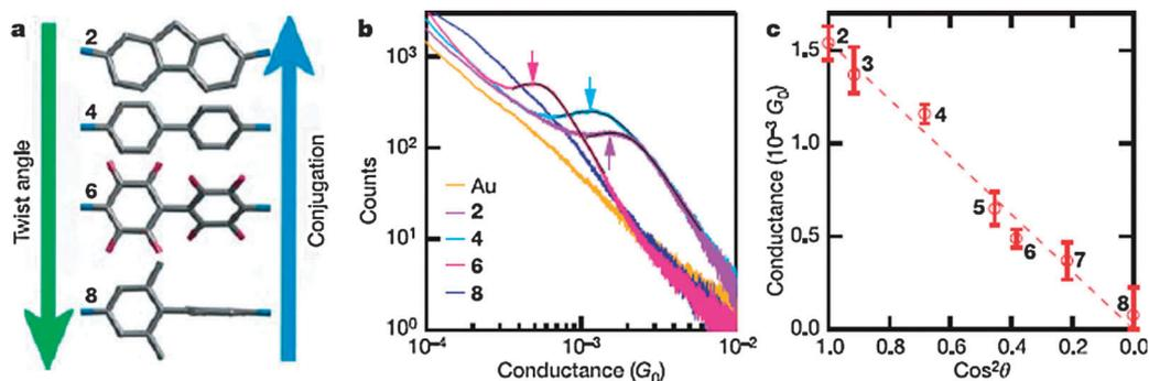
**Fig. 3** Single molecule conductance for diaminobiphenyl derivatives as a function of dihedral angle. (a) Relationship between twist angle and conjugation for four of the structures studied; (b) examples of histograms obtained from the break junction technique; (c) observed single molecule conductance dependence on twist angle. Reprinted with permission from ref. 32.
