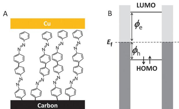
**Fig. 6** Schematic of a carbon/azobenzene/Cu molecular junction (A) and its associated energy levels (B). Dark shading in B represents filled states in the metallic contacts, while light shading indicates empty states.  $\phi_e$  and  $\phi_h$  are the energy barriers for tunnelling by electrons and holes, respectively.  $E_f$  is the system Fermi level. Adapted with permission from ref. 72.
