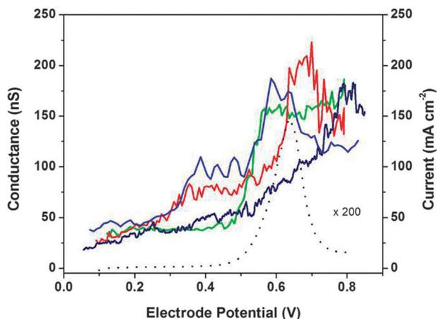
**Fig. 4** Four successive scans of the conductance (at 0.1 V) of a ferrocene derivative while the molecule's redox potential was scanned between 0 and +0.8 V relative to a reference electrode in solution (solid lines). The dotted curve (and right-side Y axis) is a conventional voltammogram of the same molecule dissolved in solution, showing the expected redox peak for ferrocene. Reprinted with permission from ref. 40.
