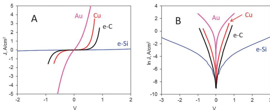
**Fig. 5** Current density–voltage curves for carbon/nitroazobenzene (NAB) MJs made by vapour deposition of the indicated top contacts on linear (A) and semilog (B) scales. Electron beam deposited silicon and carbon are denoted by e-Si and e-C, and included an additional Au layer for electrical contact. NAB thickness was 4.5 nm in all cases except e-Si, where it was 3.8 nm. Original data appears in ref. 65, 71, 72.
