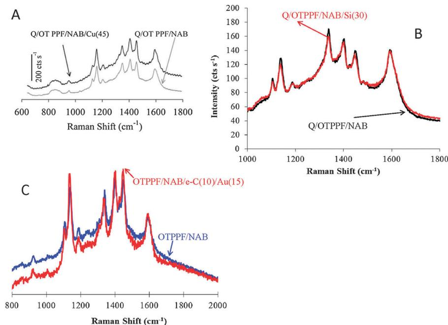
**Fig. 10** Raman spectra obtained through a partially transparent carbon substrate to which a 5 nm layer of nitroazobenzene was bonded by diazonium reduction. Two spectra are shown in each case, one taken before and one after electron-beam deposition of 45 nm of Cu (A),<sup>23</sup> 30 nm of silicon (B), or 10 nm of carbon followed by 15 nm of Au.<sup>71</sup> Figures reprinted with permission from ref. 23 (A), ref. 65 (B), and ref. 71 (C).
