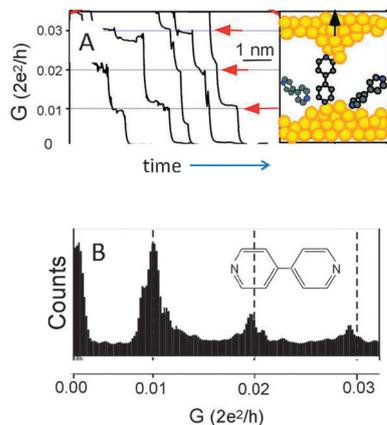
**Fig. 2** (A) Schematic of repetitive break junction technique for measuring single molecule conductance. (B) Histogram of conductance of single bipyridine molecules. Reprinted with permission from ref. 14.
